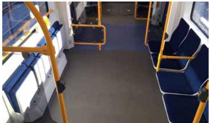
The low floor area is situated between the doors at either end of the Tram Train and offers easy wheelchair and scooter access. Other passengers must vacate the tip up seats if a wheelchair wishes to use the wheelchair area.
