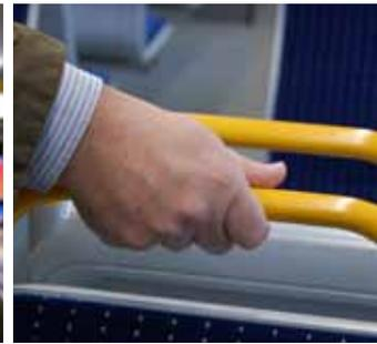
All handrails and straps are yellow making it easy to identify safe places to hold
